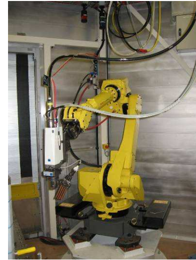
Robot Fanuc M710iC/70 Rayon d'action 2m / Payload 70 Kg
